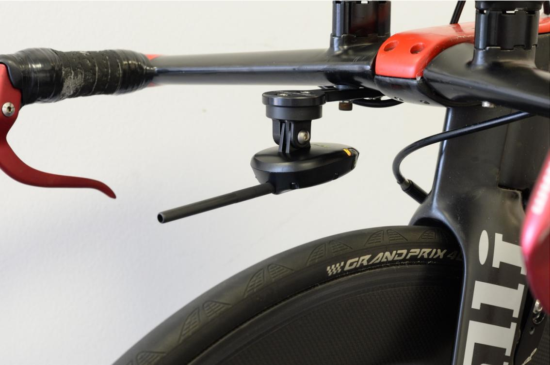
3. GoPro Grab Bag Helmet mount; double-sticky tape attaches mount to the underside of aero bars
