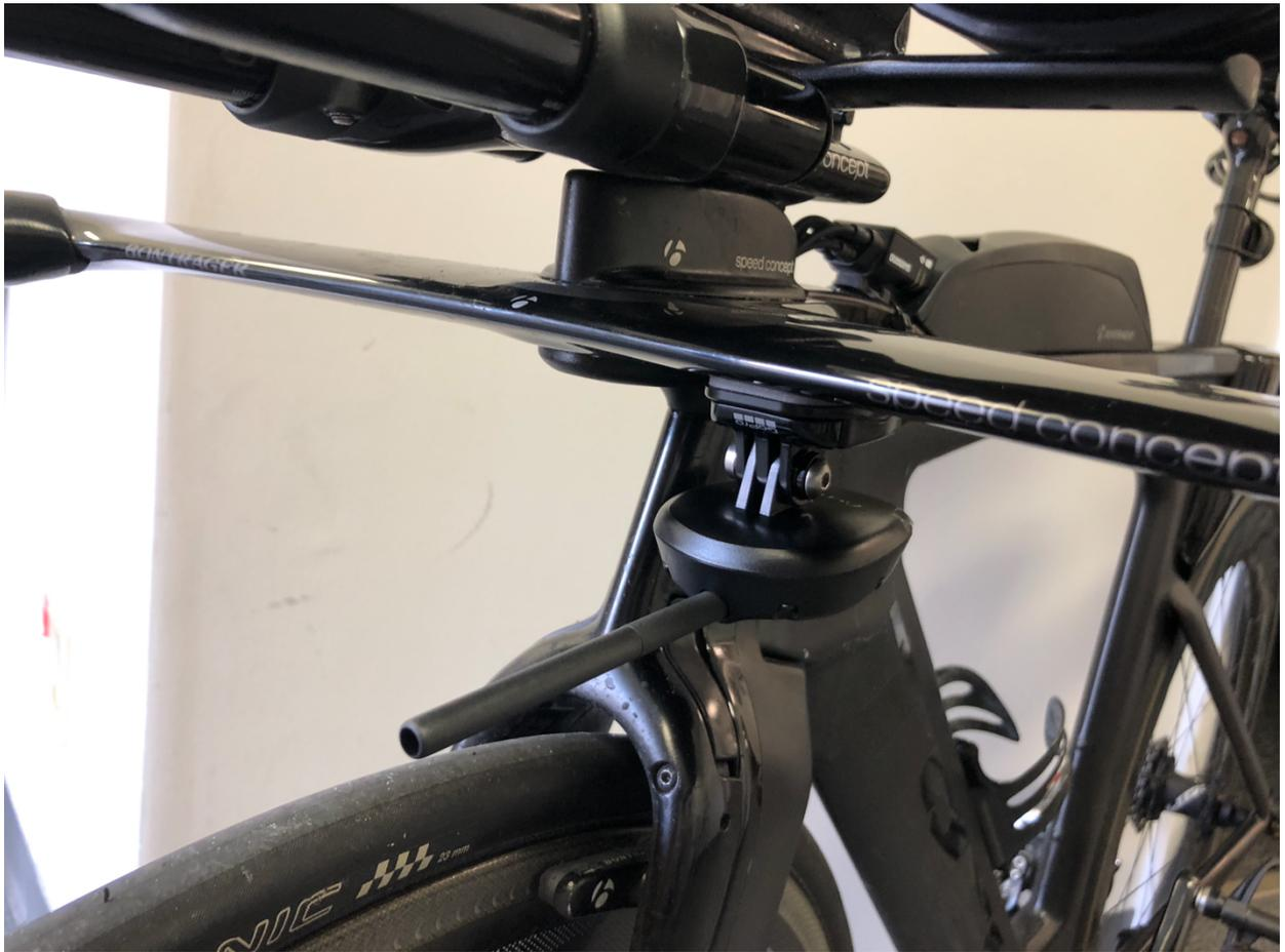
And, here is a mount system that DOES NOT WORK (because the aero bars flex)
